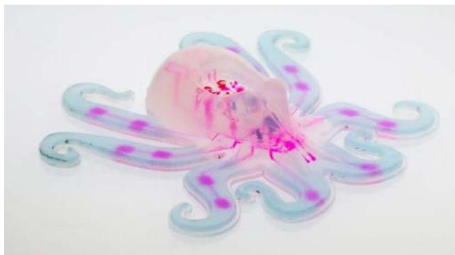
*Octobot, a small, eight-armed machine, is the first fully autonomous soft-bodied robot. Credit Lori Sanders/Harvard University*
